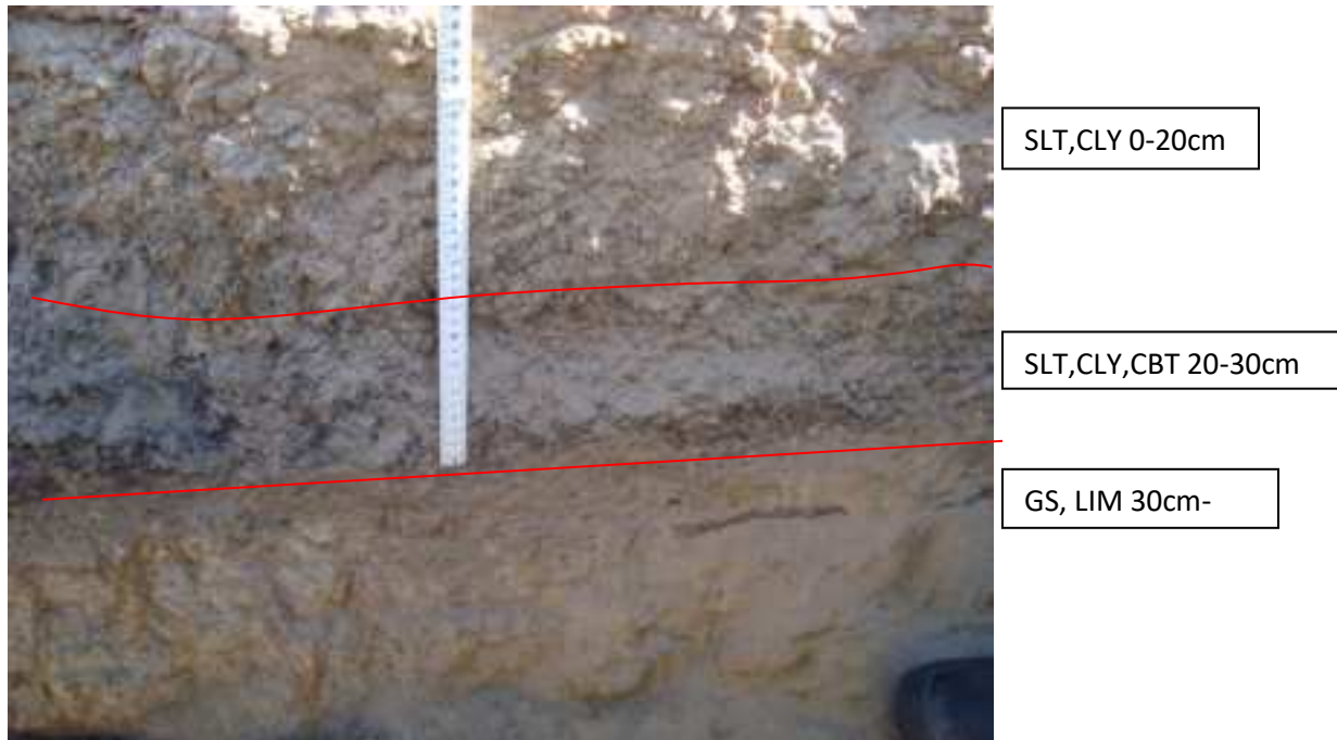
Figure 7-11. Thin carbonaceous silt and clay layer exposed in a pit at Henkries South
