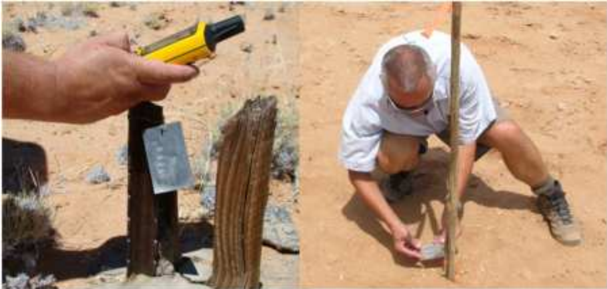
Figure 10-5. Left: example of an AOL baseline peg at 12600N. Right: A 1970's AOL drill-hole peg.
