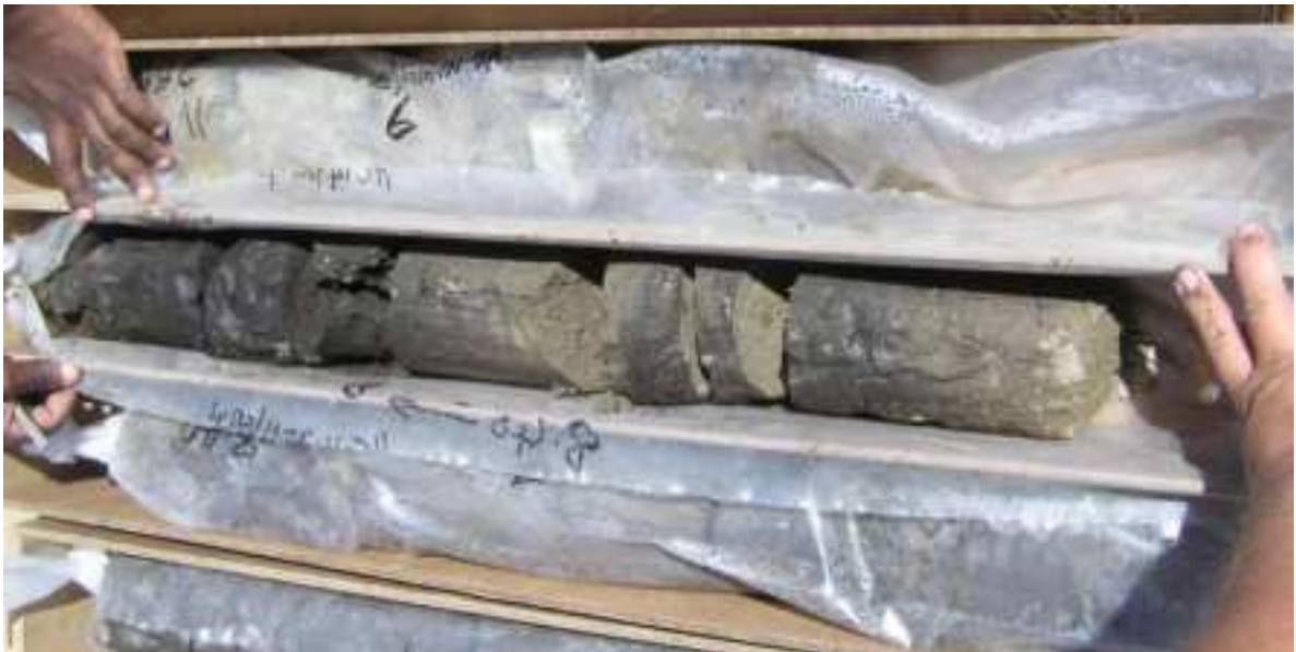
Figure 11-2. Sonic Core from Henkries Central. Clay with calcrete nodules with gradational contact over grey-black carbonaceous earth.
