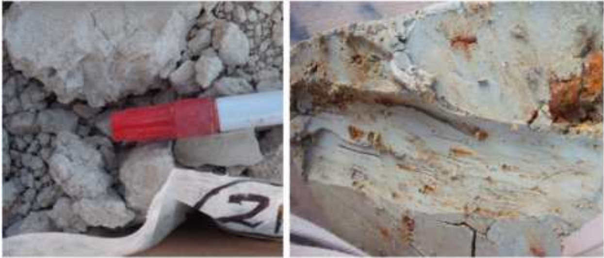
Figure 7-5. Left: massive calcrete. Right: clay to the same scale, with iron oxide
